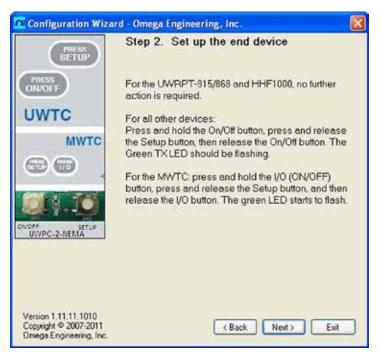
Figure 4-6. Setup The Transmitter Screen
