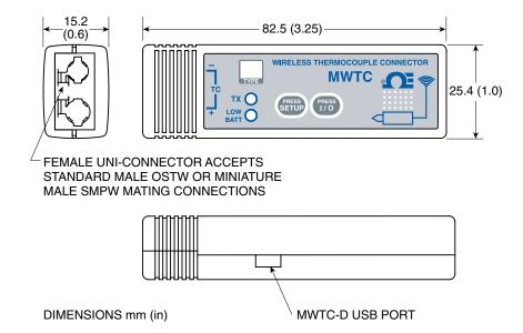
Figure 4-1. MWTC Overall Dimensions
