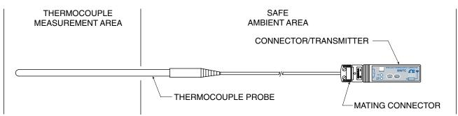
Figure 4-16. Recommended Thermocouple Placement
