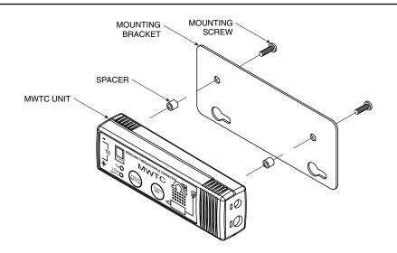
Figure 4-13. Mounting Bracket Installation
