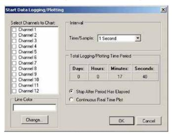
Figure 3-16. Start Data Logging/ Plotting Screen
