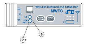
Figure 6-3. Transmit and Low Battery Lights
