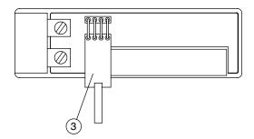
Figure 4-2B. Transmitter Programming Connector with Cable Installed
