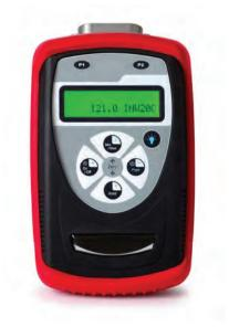
The Smart Manometer products are microcontroller based pressure sensing devices used to directly measure pressure. Differential, Gauge, Absolute and Wet/Wet pressure sensors are supported (see Specification section for supported types and pressure ranges). Pressure can be displayed in selectable engineering units of measure.
