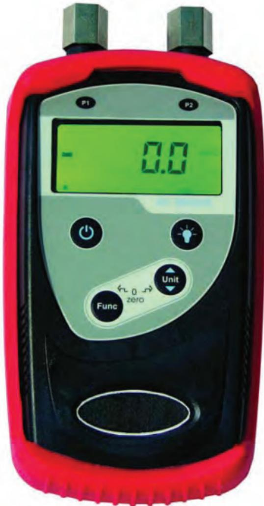
This Digital Manometer handheld instrument is a microcontroller-based sensing device used to directly measure pressure of clean, dry, non-corrosive gases. Differential, Gauge and Absolute pressure sensors are supported up to 100 PSI. Pressure can be displayed in selectable engineering units of PSI, bar, mbar, kPa, mmHg, inHg, mmH2O or inH2O.
