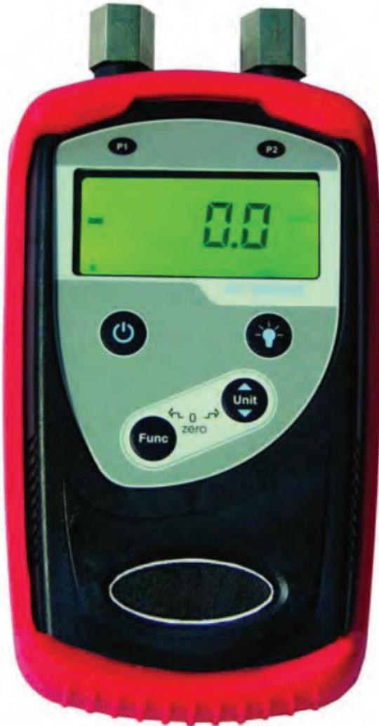
This Digital Manometer handheld instrument is a microcontroller-based sensing device used to directly measure pressure of clean, dry, non-corrosive gases. Differential, Gauge and Absolute pressure sensors are supported up to 100 PSI. Pressure can be displayed in selectable engineering units of PSI, bar, mbar, kPa, mmHg, inHg, mmH<sub>2</sub>O or inH<sub>2</sub>O.
