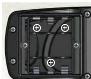
Remove the two screws located at the top center and bottom center of the battery cover by turning them counterclockwise until the fully disengaged from the DM base. Lift the cover from the back of the unit. **Do not remove the pink antistatic foam that is attached to the inside of the battery cover. This foam is necessary to properly secure the batteries under specified shock and vibration conditions!**
