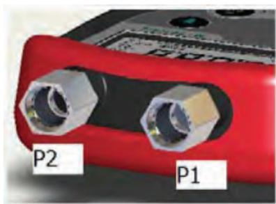
“G” Gauge and “A” Absolute models have one used pressure port, P1. P2 is used to vent enclosure/sensor to atmosphere.
