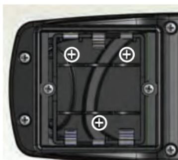
Remove the two screws located at the top center and bottom center of the battery cover by turning them counterclockwise until the fully disengaged from the DM base. Lift the cover from the back of the unit. **Do not remove the pink antistatic foam that is attached to the inside of the battery cover. This foam is necessary to properly secure the batteries under specified shock and vibration conditions!**
