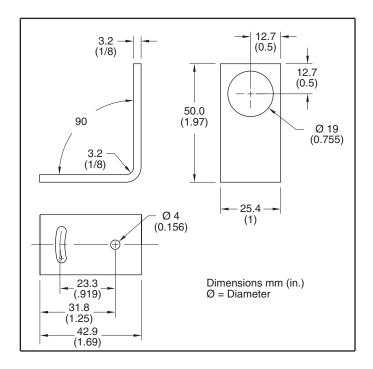
Figure 2-1. Mounting Bracket, OS100-MB
