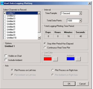
Figure 3-20. Start Data Logging/Plotting Screen
