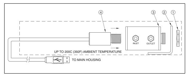
Figure 2-3. Typical Water Cool Jacket Assembly
