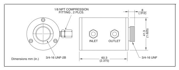
Figure 2-2. Water Cooling Jacket, OS100-WC
