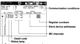
Cursor used to select a command (Used to resume command transmission from the front panel keys)
