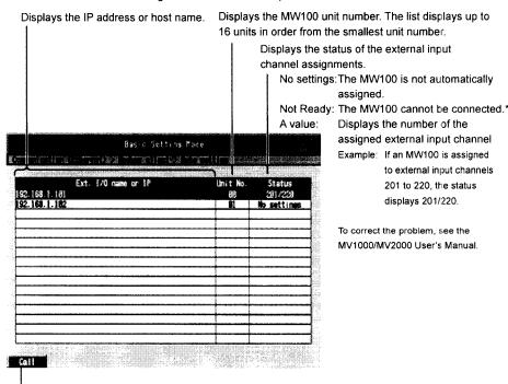
Pressing the **Call** soft key causes "--" to blink for 2 seconds on the 7-segment LED display of the selected MW100.
