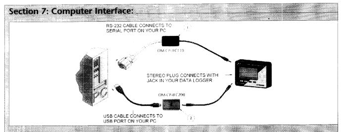
Fully insert the male connector of the IFC110 interface cable into the female receptacle of the data logger. Insert fully the RS232 connector into the Serial Port.
