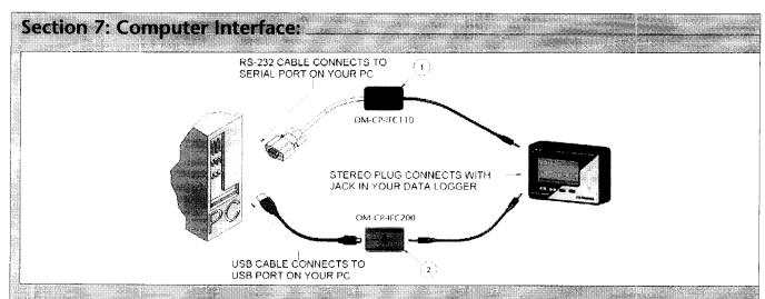
1. Fully insert the male connector of the IFC110 interface cable into the female receptacle of the data logger. Insert fully the RS232 connector into the Serial Port.
