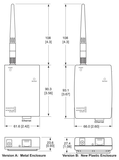
Figure 6.1 Dimensions of the Receiver
