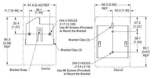
Version A: Metal Enclosure Version B: New Plastic Enclosure Figure 2.2 Mounting the Receiver
