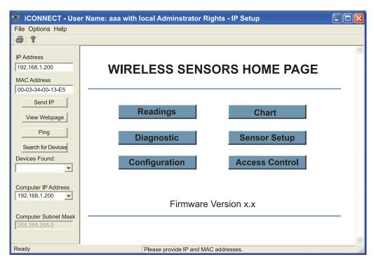
Figure 4.3 Accessing the Wireless System for Configuration
