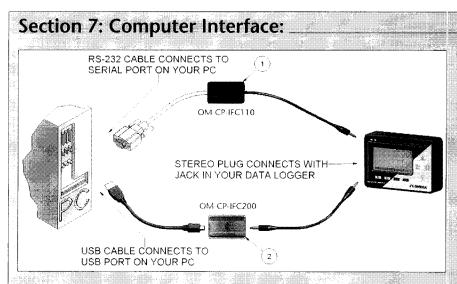
Fully insert the male connector of the IFC110 interface cable into the female receptacle of the data logger. Insert fully the RS232 connector into the Serial Port.
