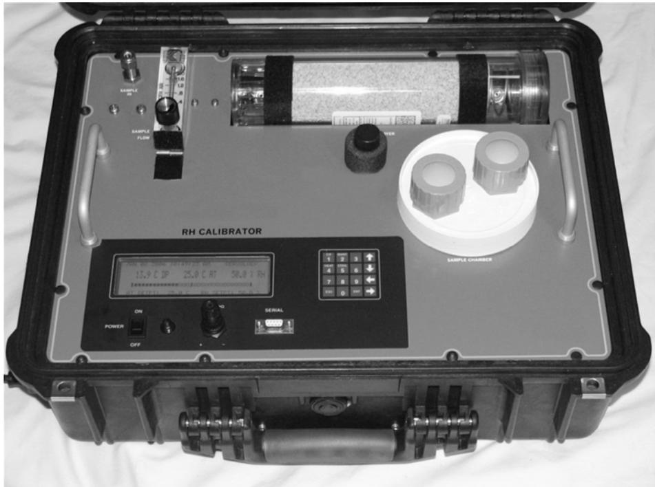
Figure 3-1 PORTABLE RH/TEMP Calibrator Panel
