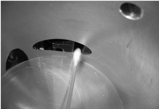
1. Remove the spin-off cover from the Sample Chamber. Notice the oval opening at the bottom of the chamber at the 3 o'clock position. Inside the opening, toward the front of the instrument and oriented vertically, the mirror is the shiny flat metal disk about  $\frac{1}{4}$  inch (0.6 cm) in diameter.
