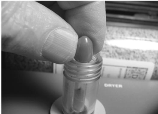
**NOTE: Whenever the RH/TEMP CALIBRATOR is moved, the saturator Shipping Plug should be installed to prevent water leakage.**
