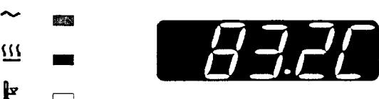
The next indicator shows when there is power to the block. When the set temperature is different to the block temperature this indicator will light. If the light is on continuously the block is getting constant power. The only exception is described under Over-Temperature Indicator. As the temperature approaches the set temperature the indicator will flash. When set temperature is reached the indicator will stay on for shorter periods.
