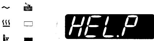
If there should, for any reason, be a sensor fault, the bottom indicator will light. The power to the block will have been switched off and the unit will begin to return to ambient even if the power light is on (the light staying on or not depends on which circuit has sensed a fault).
