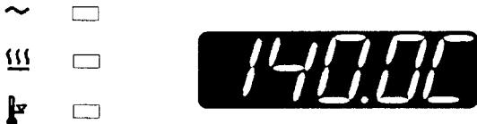
When the **SET** temperature button is held down and the **DOWN ARROW** button is pressed, the set temperature is decreased.
