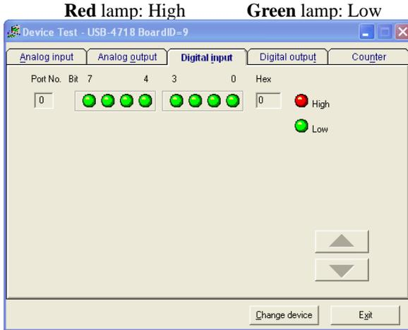
Figure 2.8: Digital Input Tab/Device Test Dialog
