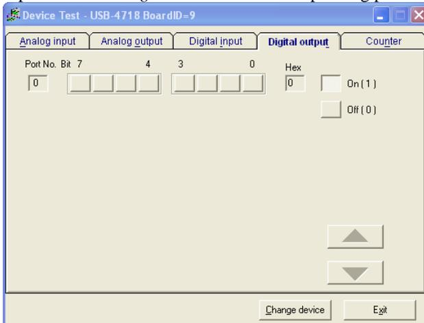
Figure 2.9: Digital Output Tab/Device Test Dialog
