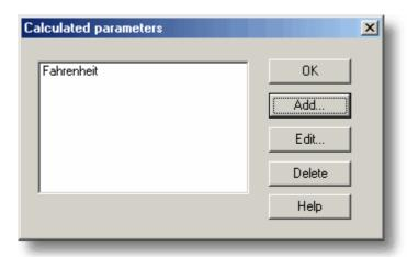
This dialog box is used to add or edit calculated parameters. Calculated parameters are readings that need some action performed on them before they can be presented as measurements. For instance, thermocouple voltage readings cannot be turned into temperature measurements without the aid of a scaling table.
