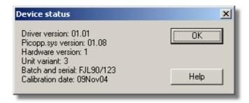
This dialog box displays the details about the ADC status. The calibration date will help you keep track of when the unit should be returned to Omega for annual recalibration (optional).
