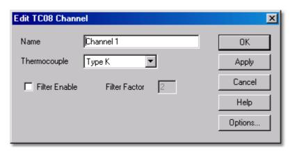
9. From the **Thermocouple** drop-down list, select the type of thermocouple you are using and click **OK.**
