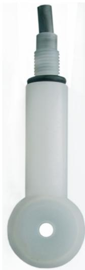
Cell Model CDE-442 is called Toroydal or Electrodeless Cell, as it does not offer electrodes. The body material could be Epoxy or PTFE, where the Toroydal nucleus (2) are located, indulging an electromagnetic field, that will generate an electrical current (called Foucault Current) proportional to the sample concentration. This type of cell is recommended for high clogging concentration and highly chemically aggressive.
