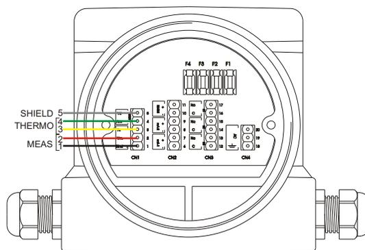
5. Verify if the cable knockouts are **firmly attached** to its respective interconnection cables. This is very important so the enclosure still offers IP-67. Sealing is crucial for a perfect performance
