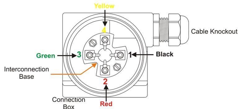
4. Electrical installation example between the equipment and the cell.
