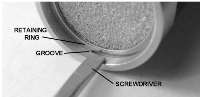
Figure 6-1 Removing the Retaining Ring
