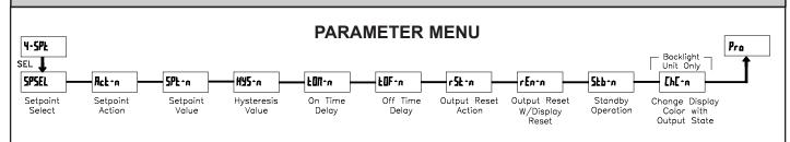
The Setpoint Output Parameters are only active when an optional output module is installed in the meter.
