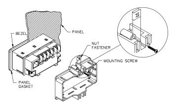
While holding the unit in place, push the panel latch over the rear of the unit so that the tabs of the panel latch engage in the slots on the case. The panel latch should be engaged in the farthest forward slot possible. To achieve a proper seal, tighten the latch screws evenly until the unit is snug in the panel (Torque to approx. 28 to 36 in-oz [0.202 to 0.26 N-m]). Do not over-tighten the screws.
