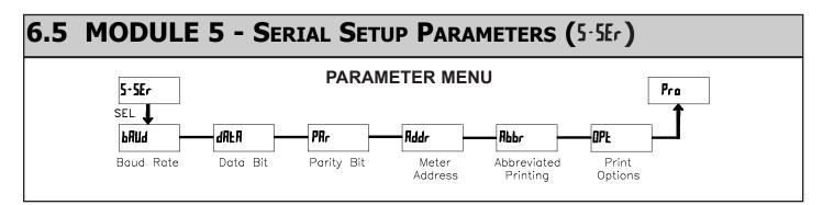
The Serial Setup Parameters are only active when the optional RS232 or RS485 serial communications module is installed in the meter. Refer to the DP6-COM bulletin for complete details on DP63000 serial communications.
