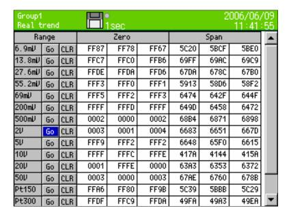
② The window which is indicate input voltage value is shown, then input the voltage value to the instrument.
