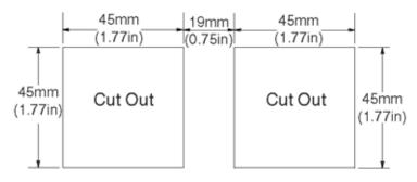
From the front of the panel, slide the housing through the cut out. The housing gasket should be against the housing flange before installing.
