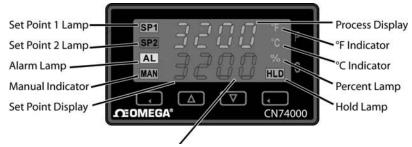
The decimal point flashes when Self-Tune is operating. Keys are illuminated when pressed. Key functions are as follows:
