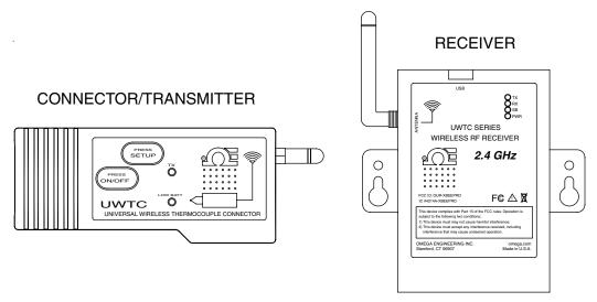
Figure 1-7. System Components
