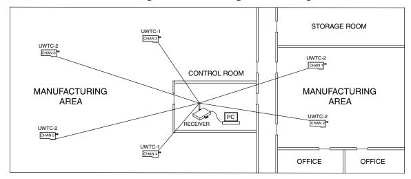
Figure 6-5. Determining Maximum Range
