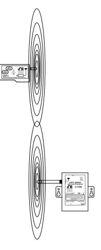
Figure 6-8. Vertical Antenna Placement
