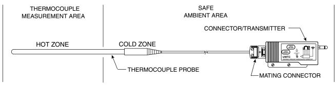
Figure 4-15. Recommended Thermocouple Placement
