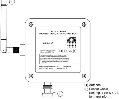
Figure 4-1B. Thermocouple/RTD Connector (UWTC-2-NEMA, UWRTD-2-NEMA)
