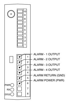
Figure 5-8. Alarm Output Connections
