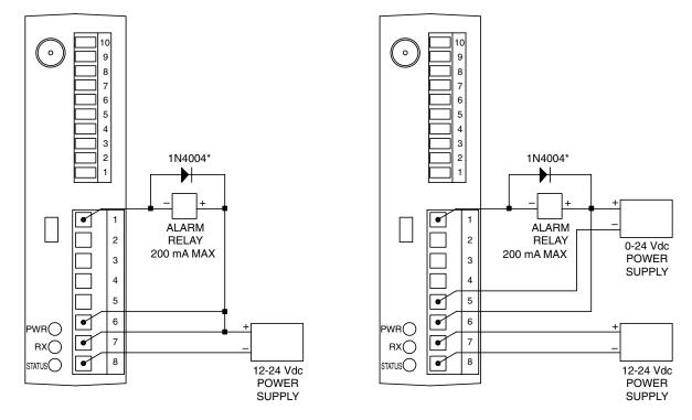
Figure 5-12. Alarm Example, System Powered
