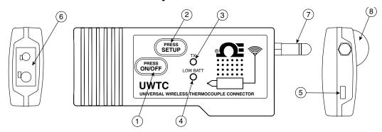
Figure 4-1A. Thermocouple Connector (UWTC-1, UWTC-2)
