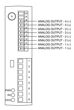
Figure 5-9. Analog Output Connections
