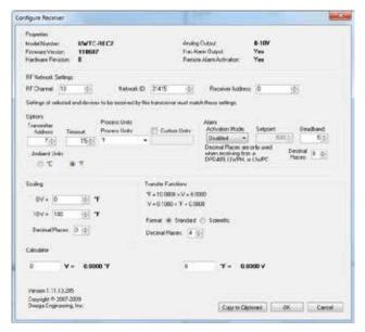
Figure 5-15B. UWTC-REC2 Setup Screen
