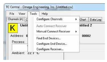
Figure 3-20. Tools Menu Tab Screen Configuration
