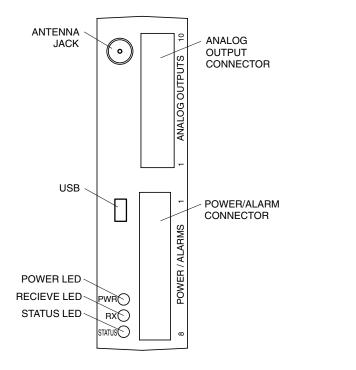
Figure 5-6. Receiver Operation - UWTC-REC4
