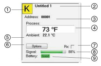
Figure 3-12. Channel Display Box Screen
