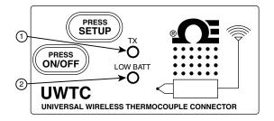
Figure 6-3. Transmit and Low Battery Lights
