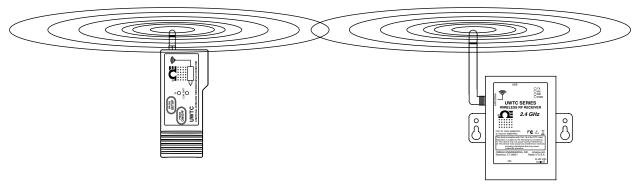
Figure 6-7. Horizontal Antenna Placement
