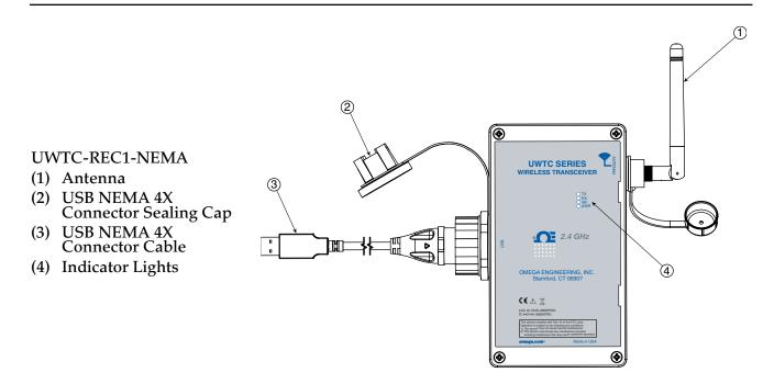
Figure 5-5A. Receiver Operation - UWTC-REC1-NEMA, UWTC-REC1-915-NEMA
