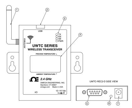
Figure 5-3. Receiver Operation - UWTC-REC2-D
