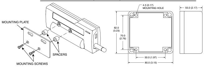
Figure 4-12A. Mounting Bracket Installation UWTC-1, UWTC-2, UWRTD-1, UWRTD-2 4.2.2 Mounting
