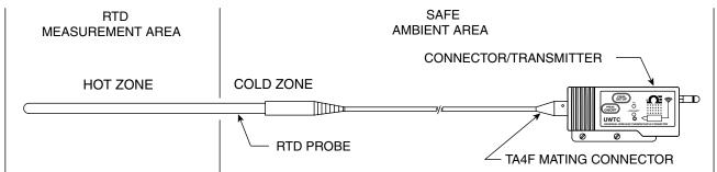
Figure 4-17. Recommended RTD Placement
