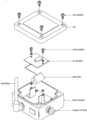
Figure 4-18B. Battery Placement UWTC-2-NEMA, UWRTD-2-NEMA
