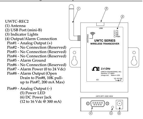
Figure 5-2. Receiver Operation - UWTC-REC2
