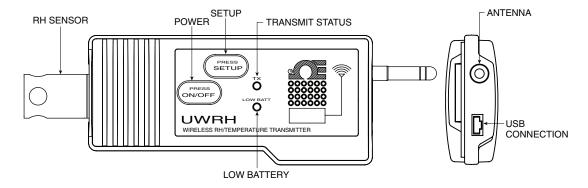
Figure 1A. Main Transmitter Operations, UWRH-2
