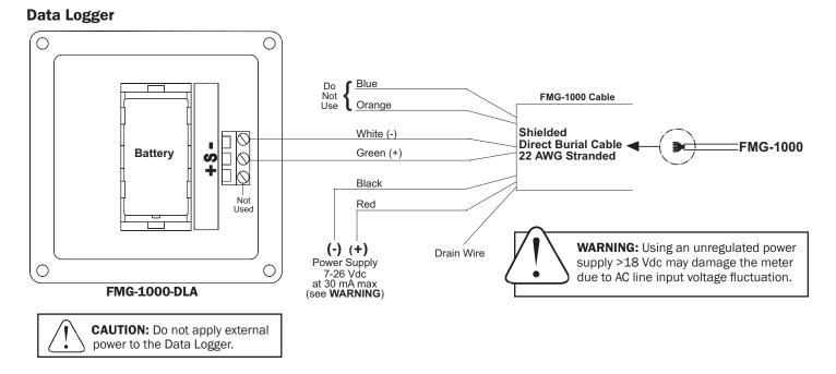
The **FMG-1000** requires a power source of 7 to 26 Vdc at 30 mA max (see **WARNING**). The same cable that provides power also serves as a pulse output if needed for remote reading, data logging, signal conversion, or telemetry.
