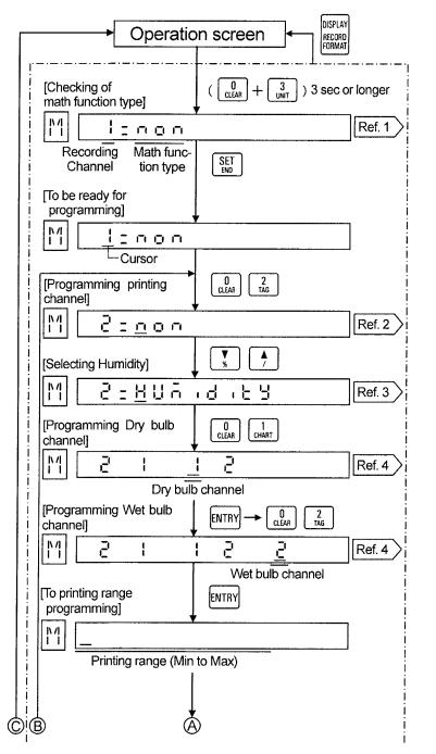
Checking of Ref. 1 other channels You can check the math function type of other channels. Press to change or channels.
