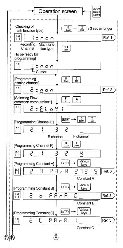
Checking of other channels You can check the math function type of other channels. to change Press or channels Ref. 2 > Channel digit In AH3000 series multi-point type, a channel is programmed by two digits (06/12/24).Constants of A, B, C and D -1. Not-used constants For the not-used constant (B), program it to '0. 2. Programming of constants (1) 5 digits or less including a (2) Down to three decimal places 3. For FloW3, the constant D is not existed.
