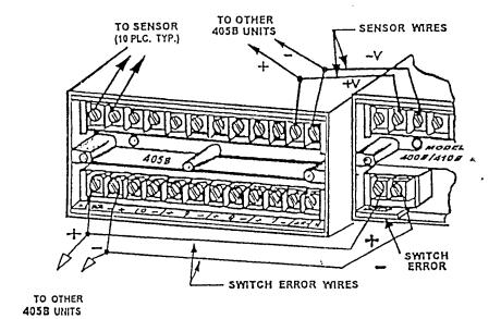
FIGURE 2.11A. INTERFACE DETWEEN MODELS 400B / 410B AND 405B
