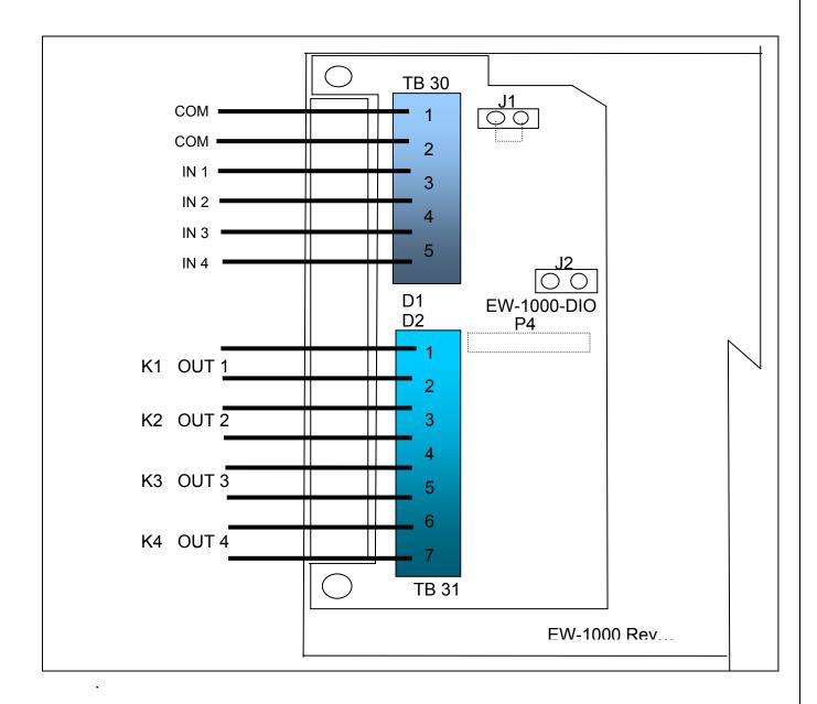
**Option 2 DIO: "SEL.OP2"** First select the operating mode for "Setpoint", "Over/Under", "Manual or Auto Batch". After setup, the parameters for the selection are entered from the weighing mode.
