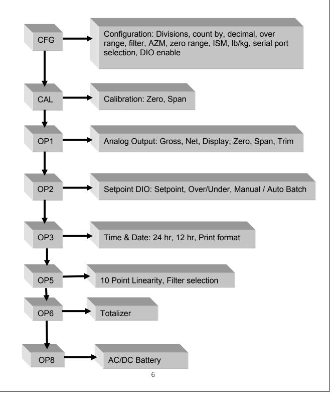
**CONFIGURATION: "SEL.CFG"** Use Zero to enter the menu and step to each category, Gross/Net to select parameters. Print to return to menu selection.
