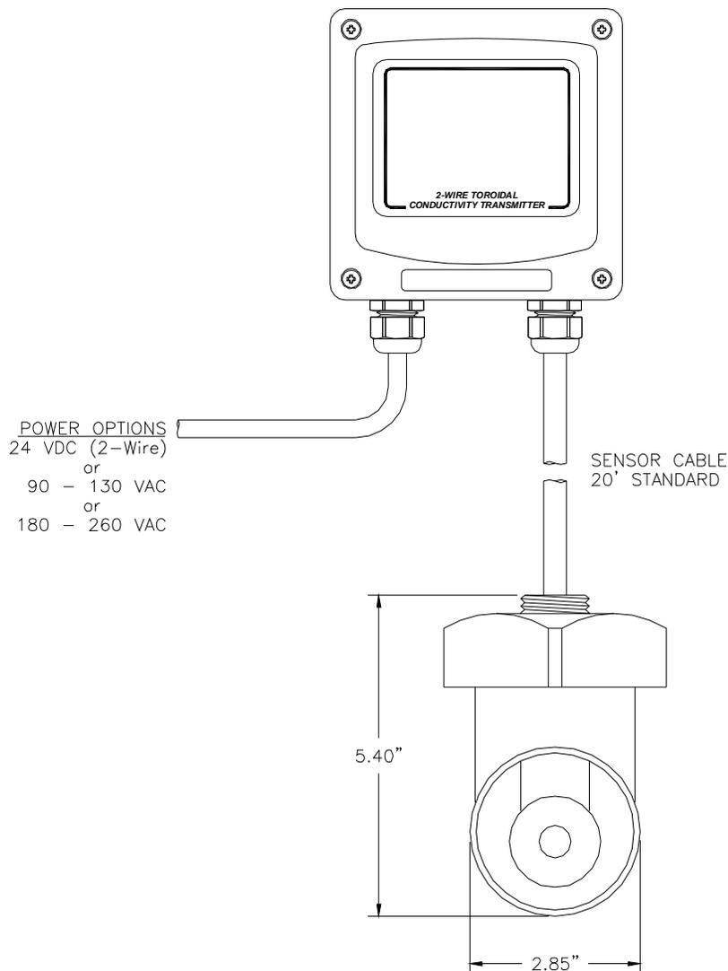
**Figure 3-2 Sensor Mounting - Tee Assembly**
