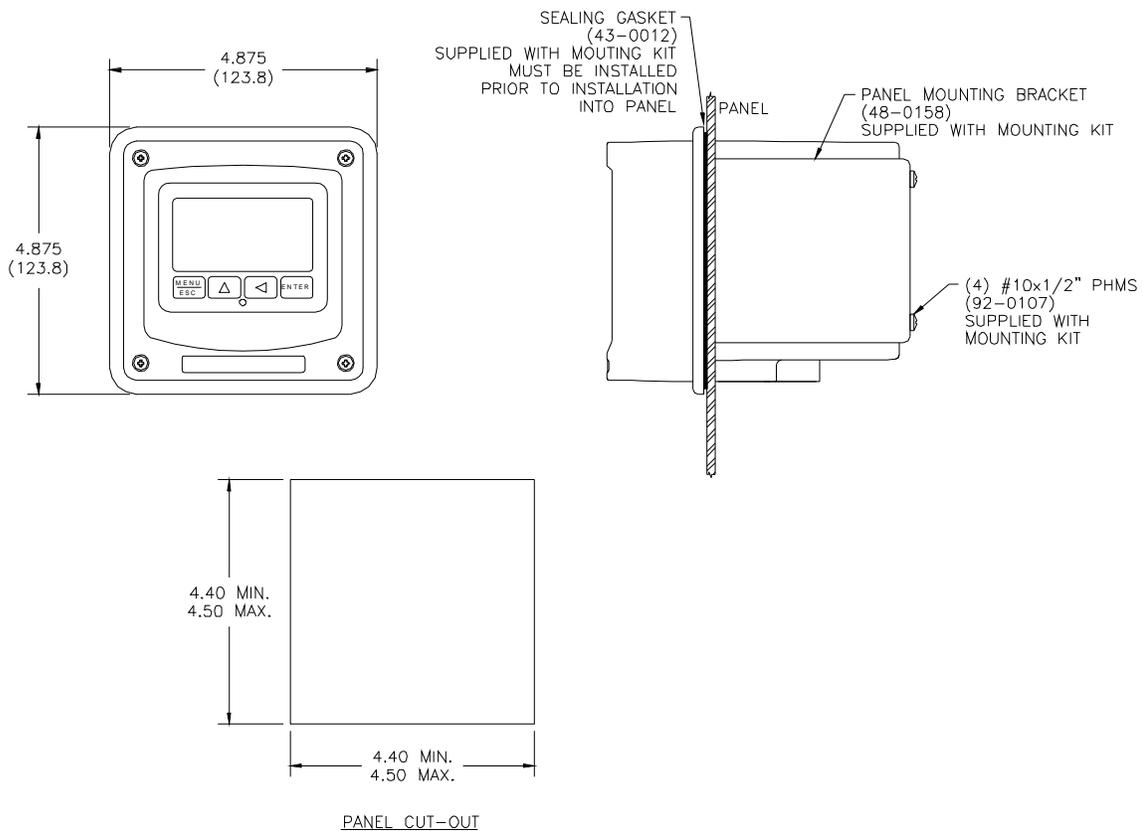
**Figure 2-6 115/230 VAC Panel Mount and Cut-out**
