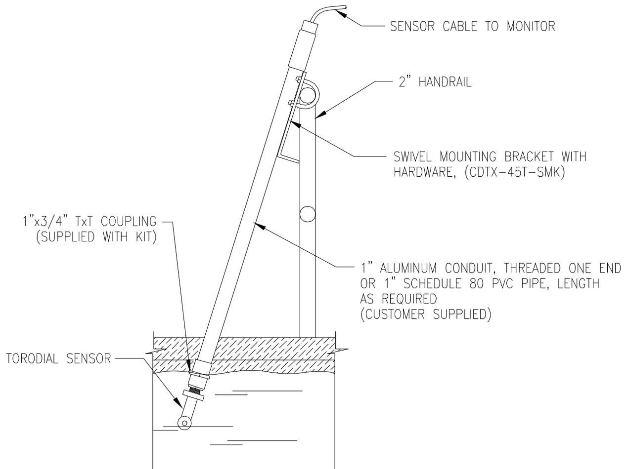
**Figure 3-3 Submersible Sensor Mounting Assembly**
