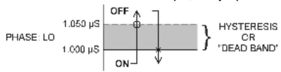
When value rises to  $\geq 1.000 \mu\text{S}$ , relay opens.
