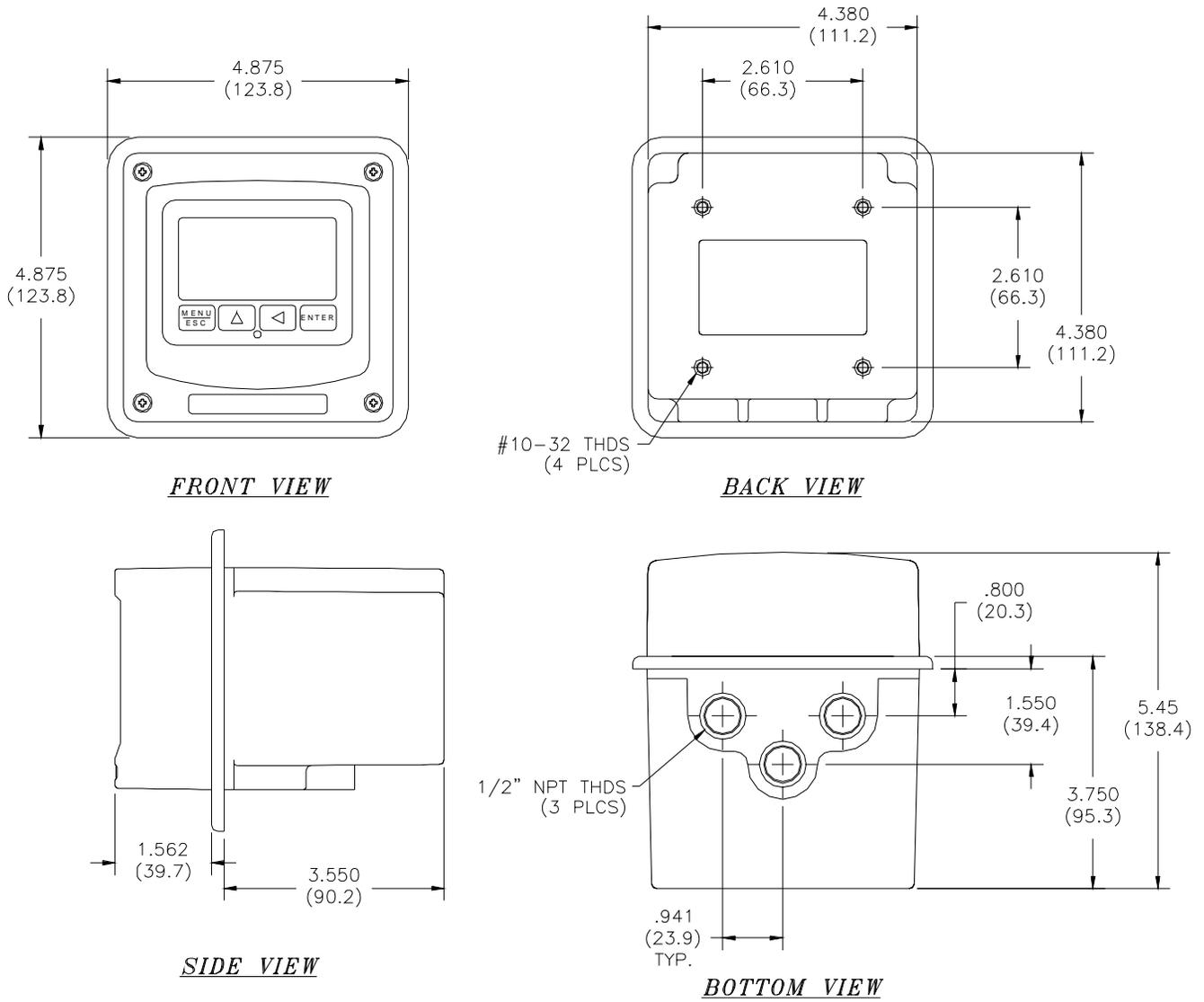
**Figure 2-1 CDTX Enclosure Dimensions, AC Powered Units**
