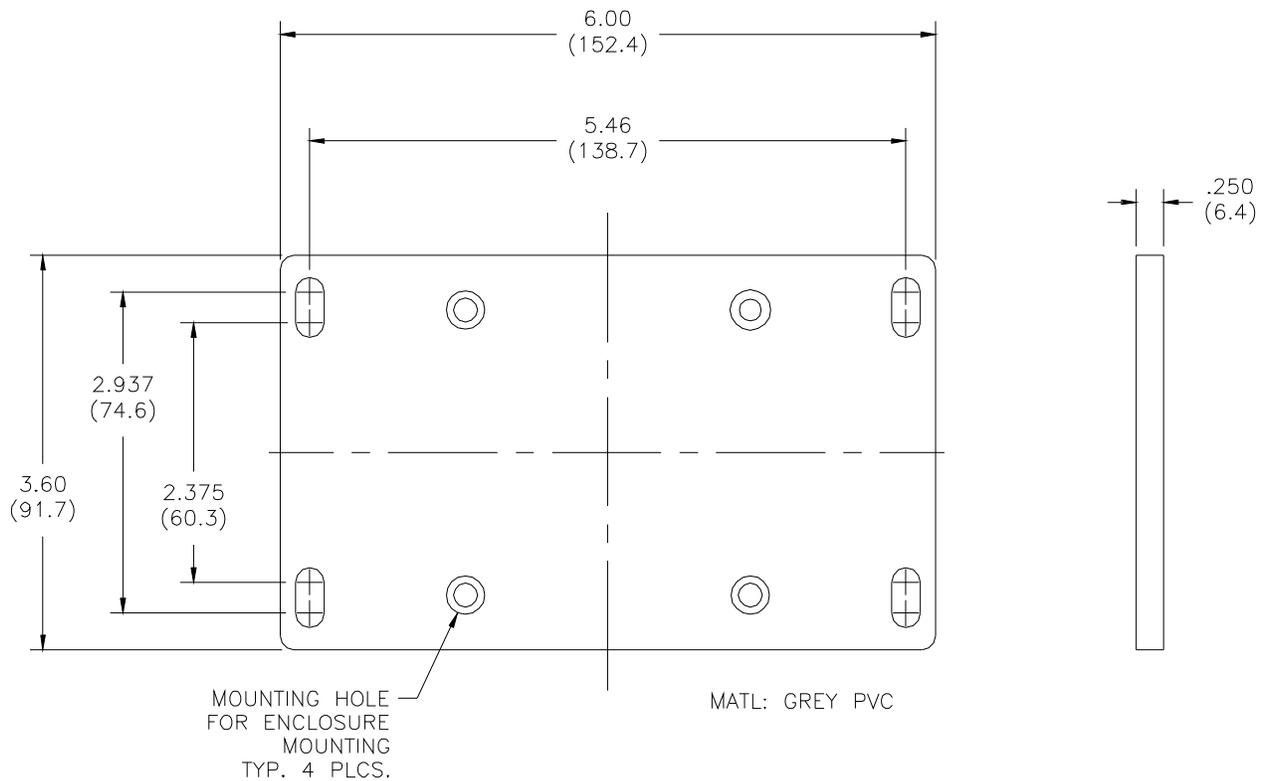
**Figure 2-3 Wall or Pipe mount Bracket**
