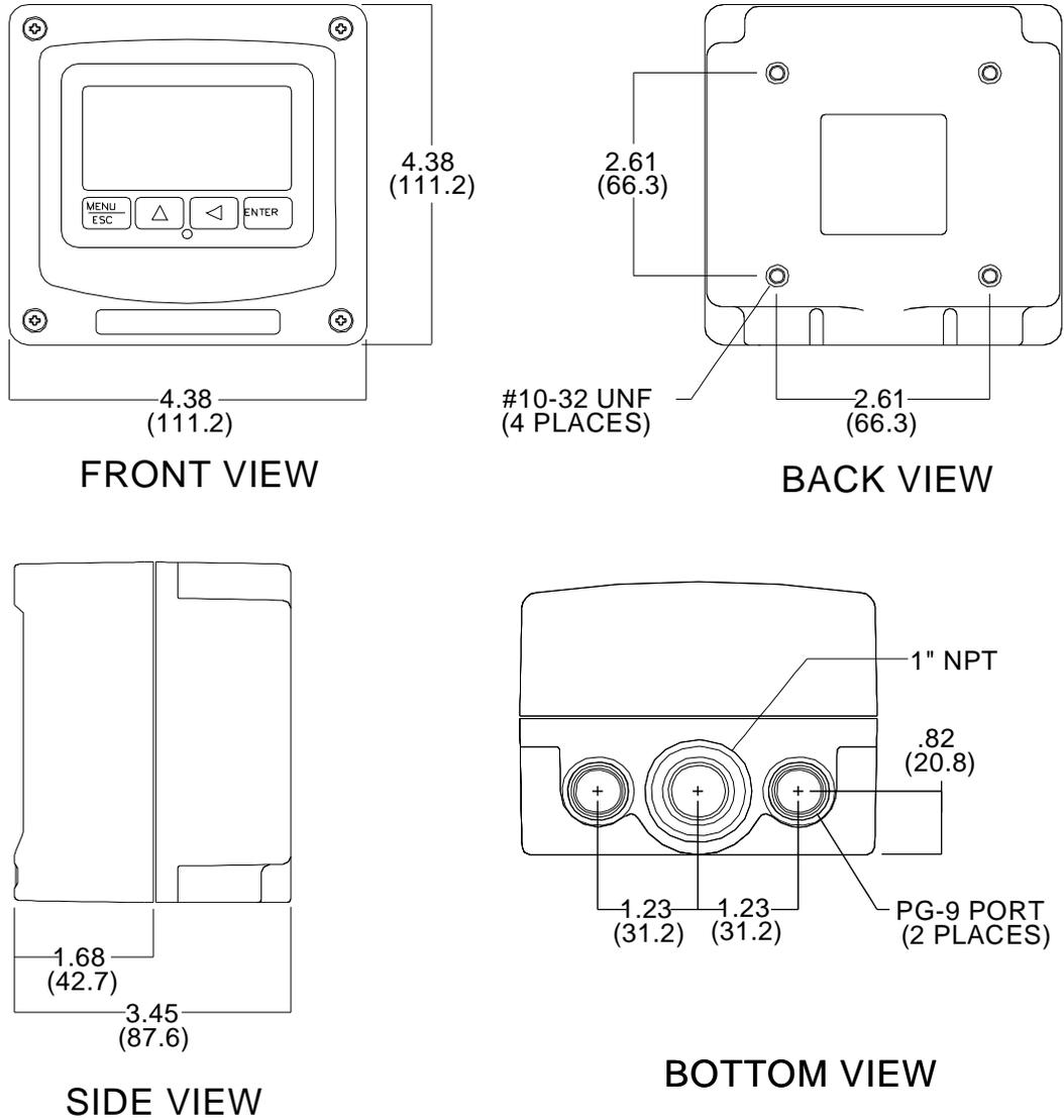
**Figure 2-2 CDTX Enclosure Dimensions, 2-Wire and Battery Units**
