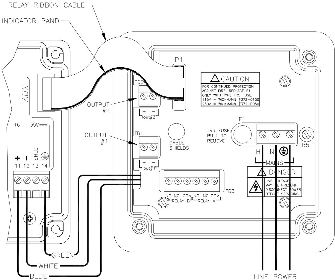
**Figure 4-2 Line Power Connection**
