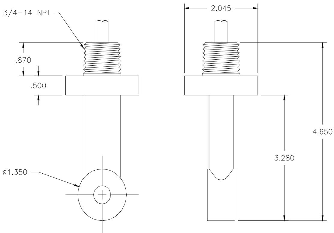
**Figure 3-1 Submersible Sensor Mounting Assembly**
