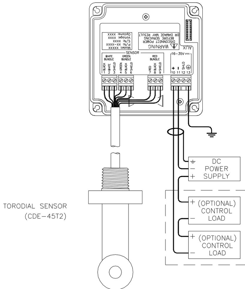
**Figure 4-1 Loop-Power Connection, CDTX-45T Transmitter**
