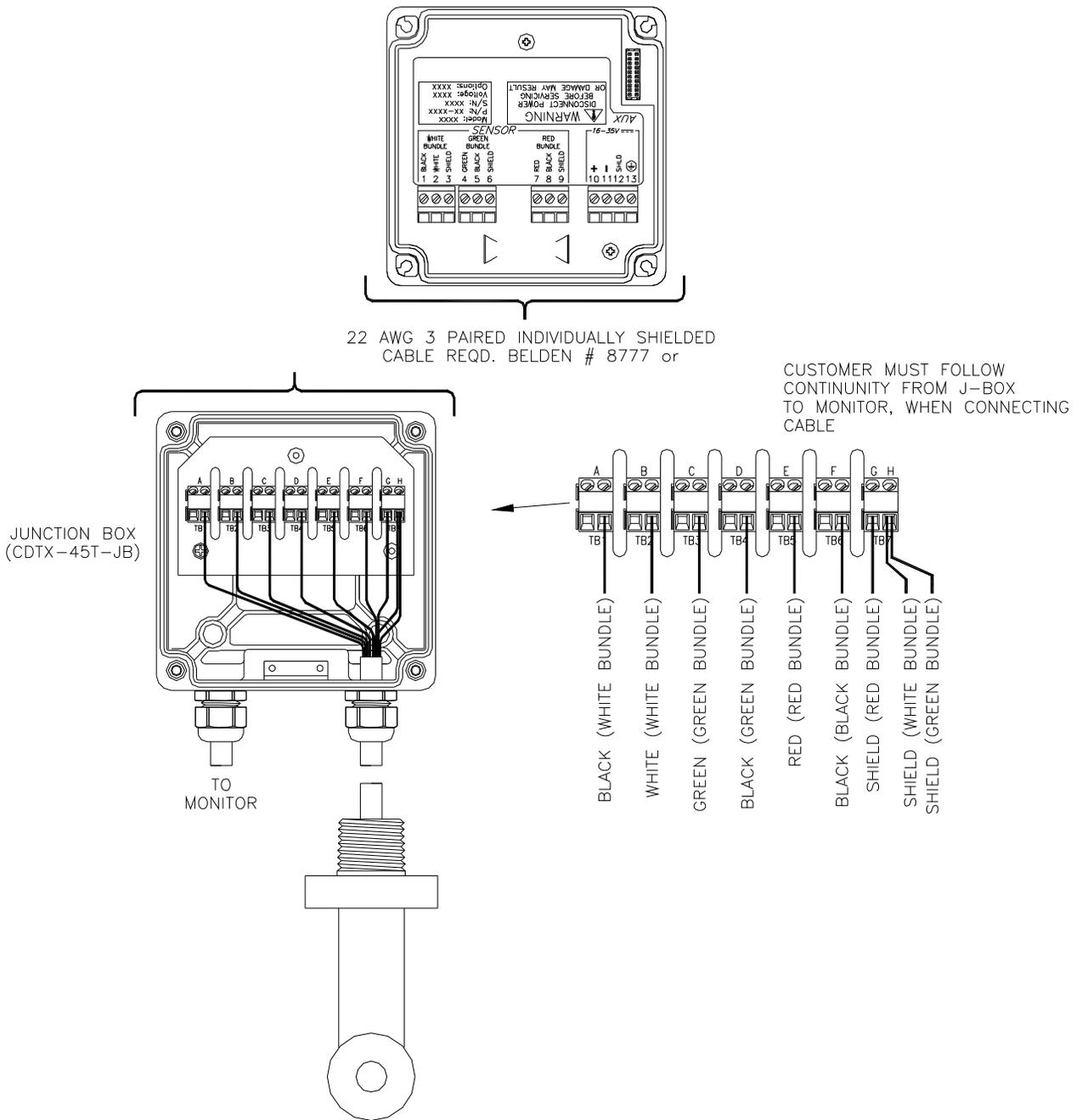
**Figure 4-5 Junction Box Wiring**
