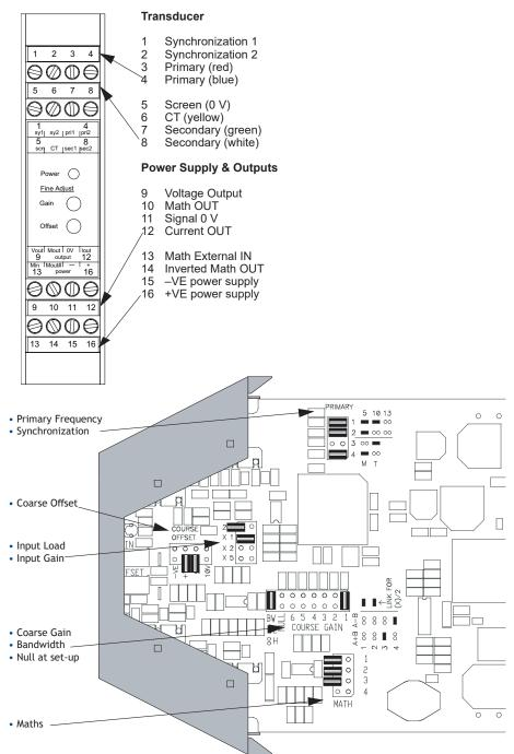
Terminals 5, 11, and 15 are internally connected but, for best performance, they should be treated as separate terminals.
