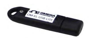
This low cost data logger measures and stores up to 4,080 temperature readings over a -10 to +50  $^{\circ}$ C (+14 to +122  $^{\circ}$ F) measurement range with a fixed 30 minute sample rate and a battery life of 1 month continuous use.
