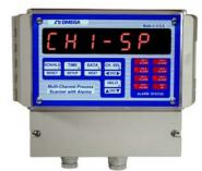
b) The second method of displaying deviation is by selecting the 'dSP dEN' option when programming the Display Option during the SYS Setup. If this method is selected, the display will scan through all the active channels and display their deviation. The display format is 'd2 1234' (d stands for deviation).
