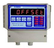
After pushing **SETUP** key at the completion of Setup For Low Scale, the display will briefly read '**OFFSEt**', and then show the present Offset value. The active digit will be flashing. Use the ▲**DIG**▼ key (as described in Setup For High Scale) to enter a desired OFFSET value. After the desired OFFSET value is displayed, push **SETUP** key to go to Tare setup.
