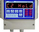
To select another channel for display during hold mode, push the **CH. SEL** key. Each push will increment the channel number. The display will first show the channel number (e.g. **'CHANEL 2'** for channel # 2) followed by the process variable in the form **'0.123 PSI'**. When channel selection is initiated using the **CH. SEL** key, the unit starts with channel #1 and steps thru to channel #7 with each push of the key.
