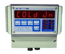
**NOTE 2:** Cold-junction temperature is the temperature of the connector that connects the thermocouple to the unit. This temperature is usually higher than ambient temperature, particularly after the unit has been powered for some time. This is due to the heat generated by internal electronics of the unit. For precise calibration, measure the temperature at thermocouple connector and then adjust Cold-junction reading.
