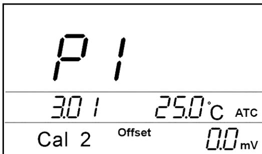
“P1” , the LCD displays as left chart. Press< M+/□>short key to display zero potential of the pH sensor (Offset) mV value、Slope value alternatively. Information displayed in left chart : the calibration date of PH sensor is 1<sup>st</sup> of
