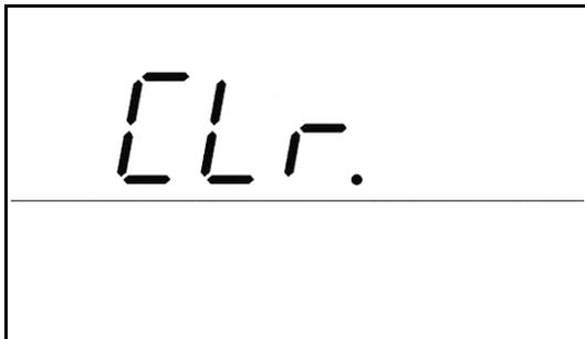
When the instrument memory is full, will not store the measurement information; or the information stored is not needed anymore, clear the memory is needed. Under the measurement mode ( pH or mV measurement ) , press<
