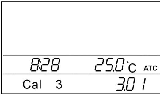
instrument reminds you 1 point calibration is finished, do you want to proceed 3 points calibration? If only 2 point calibration needed, press “READ” to exit calibration process, switch to pH measurement mode. If the 3 points
