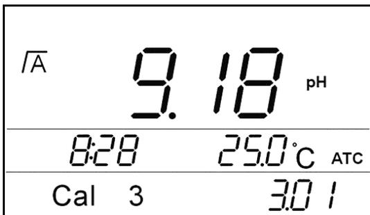
After 2 point calibration, LCD displays as above chart ( “Cal3” flashes), immerse the electrode into third standard buffer solution(e.g. PH9.18 Buffer), shaking the vessel for few minutes, wait for second, press “CA L” ,
