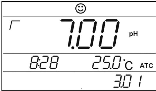
Under pH measurement mode, immerse the sensor into the sample after rinsing with distilled water, shaking the vessel few minutes, if the instrument has not been set to auto ending function, LCD will display “√” icon if the
