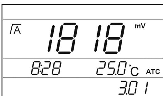
“READ” key( short key ) ,when the LCD display “√A” auto ending function icon, the instrument will block the measurement value, the value could be read. In left chart, the date is 1<sup>st</sup> March, time is 8 o'clock 28 , the sample
