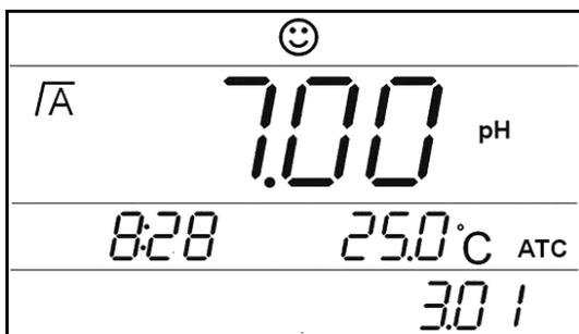
icon, the instrument will block the measurement value, the value could be read. In left chart, the date is 1<sup>st</sup> March, time is 8 o'clock 28 , the sample temperature is 25.0°C , automatic temperature compensation ( ATC ) , auto
