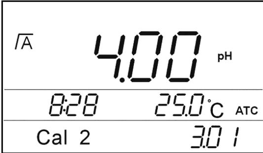
After 1 point calibration, LCD displays as above chart ( “Cal2” flashes), immerse the electrode into standard buffer solution, shaking the vessel for few minutes, wait for second, press “CA L” , the instrument will recognize which buffer
