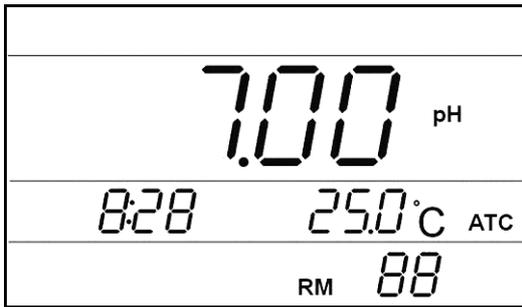
In below chart, measurement value number is 88 , 7.00pH , measurement time 8:28( display measurement date and measurement time alternatively ) , sample temperature is 25.0°C ( ATC ) .
