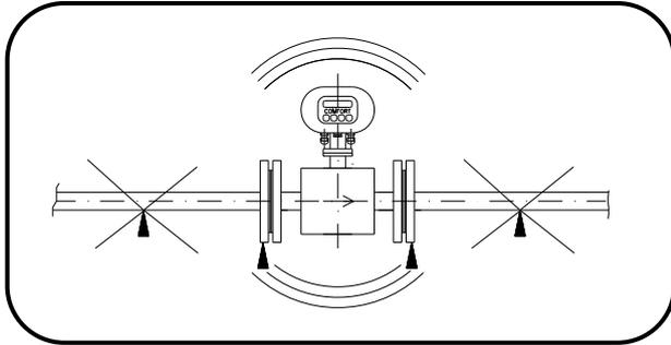
Undesirable sensor vibrations
