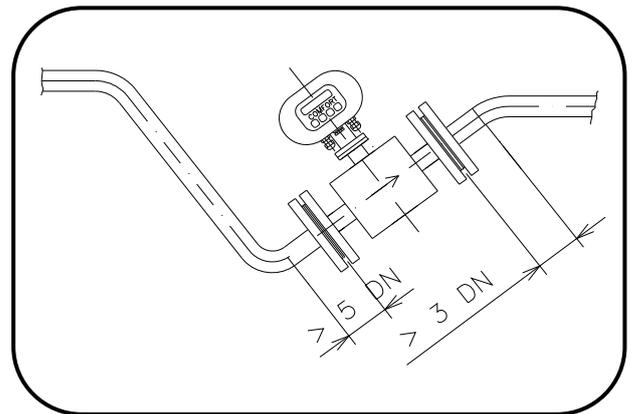
Permanent flooding of sensor
