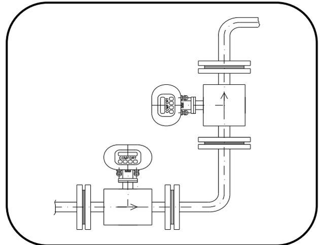
Sensor mounted in a vertical position
