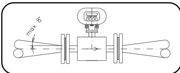
In the case where the pipeline nominal size is bigger than nominal size of flow meter, it is necessary to use conical reduction with the maximum slope  $15^\circ$ . In the case of bi-directional flow, conical reduction must be installed on both sides, both with minimum straight piping 5 DN. In the case of horizontal installation, eccentric reduction must be use to prevent bubbling.
