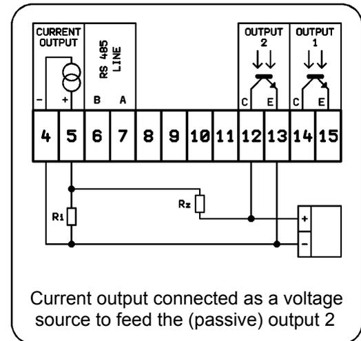
The output voltage for the associated equipment is defined as the voltage drop on resistor R. It holds:  $U = I R$ .
