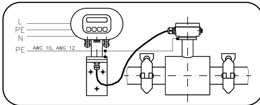
With a remote version, it is recommended to electrically connect flow sensor with electronics housing box with conductors AWG10 or AWG12 to assure stabilization of the electric potentials.
