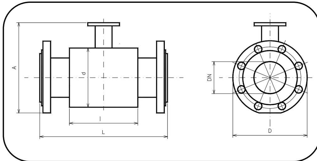
Sensor dimensions for various rated diameters Line size (DN)
