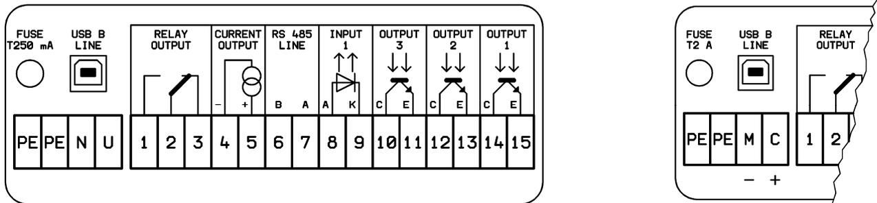
Examples of labels showing power supply (line voltage or 24VDC source) and meter signal interconnection
