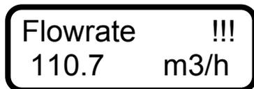
The flow-rate display image with the zero setting effective
