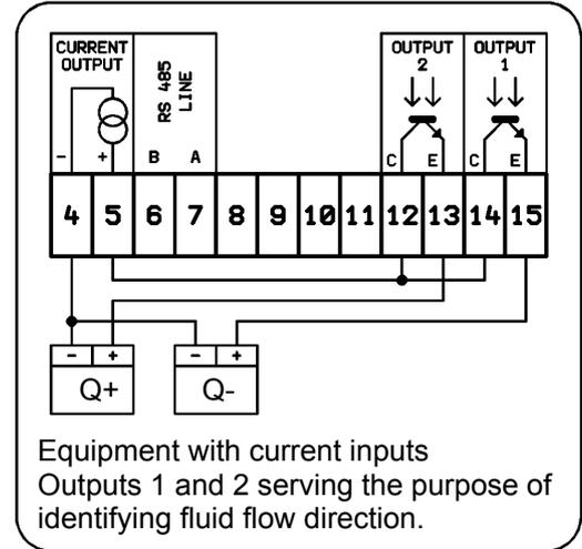
Multifunctional outputs programmed to identify the fluid flow direction and negate the flow direction, will divide the analog output operated in the “Absolute Flow Rate Value” mode into two outputs, one for each flow direction.
