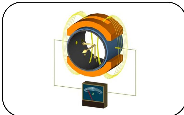
As the magnetic flux density and distance between the electrodes are constant, the induced voltage is proportional to the liquid flow velocity in the tube. The value of the volume flow rate can then be readily determined as a product of the flow velocity and square section of the tube,  $Q = v \times S$ .
