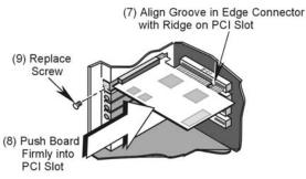
Installing a DaqBoard/500 Series Board
