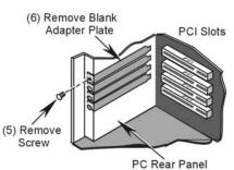
Removing a Blank Adapter Plate
