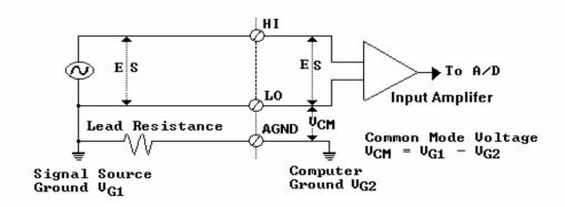
**Differential Configuration for Grounded Sources**
