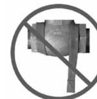
C.) Incorrect Installation: Heating tape hanging free from the surface
