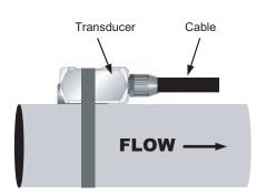
Figure 2.2 Top View of Pipe operating range of the meter. Down stream from pump or orifices, etc., locate at least 20 diameters. See **Table 2.1**
