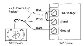
Input designed for current sourcing (PNP) devices
