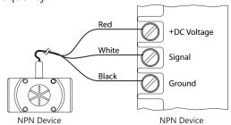
Input designed for current sinking devices (NPN)
