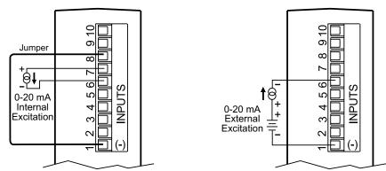
Figure 2.6 Process Current Wiring Hookup (Internal and External Excitation)
