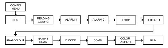
Figure 3.2 Flow Chart for Configuration Menu
