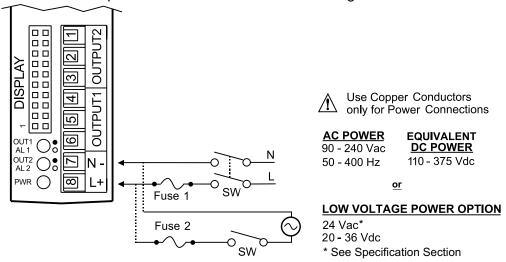
Figure 2.3 Main Power Connections
