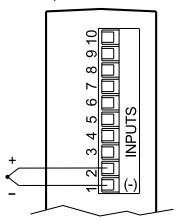
**Figure 2.4 Thermocouple Wiring Hookup**
