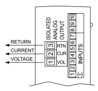
Figure 2.9 Isolated Analog Output Wiring Hookup.
