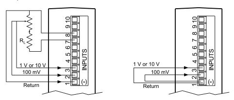
Figure 2.7 Process Voltage Wiring Hookup (with Sensor Excitation and without Sensor Excitation)
