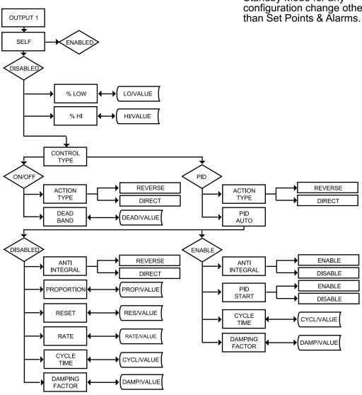
Figure 3.8 Flow Chart for Output 1
