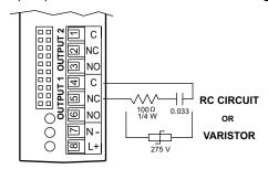
Figure 2.10 Snubber Circuits Wiring Hookup
