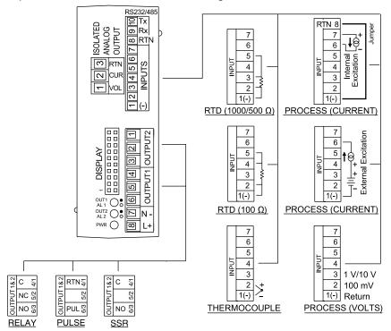
**Figure 2.2 Input and Output Connections**
