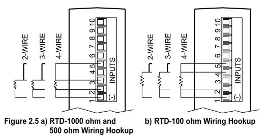
The **two-wire** connection is simplest method, but does not compensate for lead-wire temperature change and often requires calibration to cancel lead-wire resistance offset.
