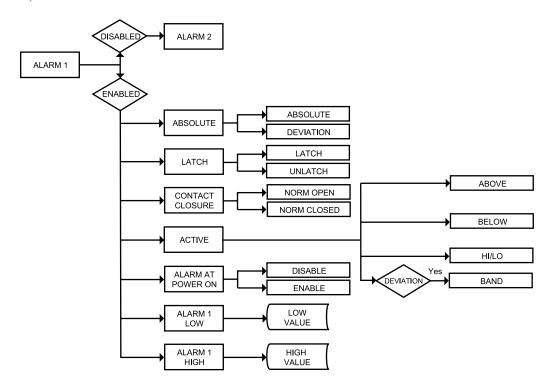
Figure 3.5 Flow Chart for Alarm 1
