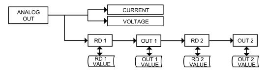
Figure 3.9 Flow Chart for Analog Output (Retransmission)
