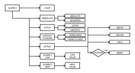
Figure 3.6 Flow Chart for Alarm 2
