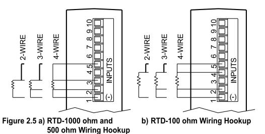
The **two-wire** connection is simplest method, but does not compensate for lead-wire temperature change and often requires calibration to cancel lead-wire resistance offset.
