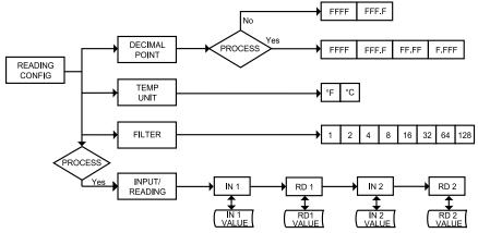
Figure 3.4 Flow Chart for Reading Configuration Menu
