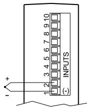
Figure 2.4 Thermocouple Wiring Hookup
