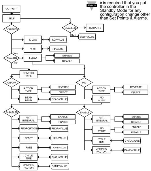
Figure 3.9 Flow Chart for Output 1
