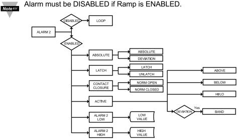
Figure 3.7 Flow Chart for Alarm 2
