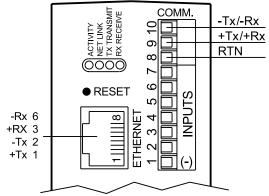
Figure 2.13 Embedded Ethernet
