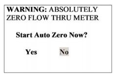
Figure **b-18**, Zero Calibration (Start)
