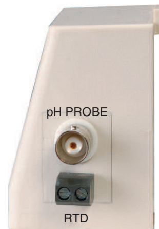
Figure 2-18. pH Probe/RTD Connections
