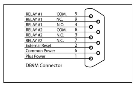
Attach the 9-pin D-connector to the module (fig. 1 & 2).
