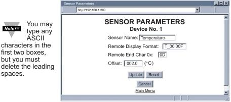
Figure 4.15 Sensor Parameters
