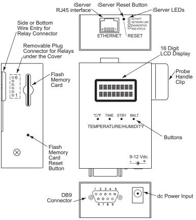
Figure 2.4 Parts of the iServer Unit
