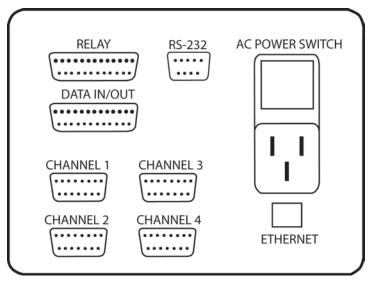
Figure **b-1**, Interface Panel for FMA14PD.
