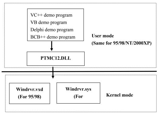
The install shield will install kernel driver, DLL driver & application demo program to system. All demo programs & DLLs are same for 95/98/NT/2000/XP. But the kernel drivers are different for different system as follows:
