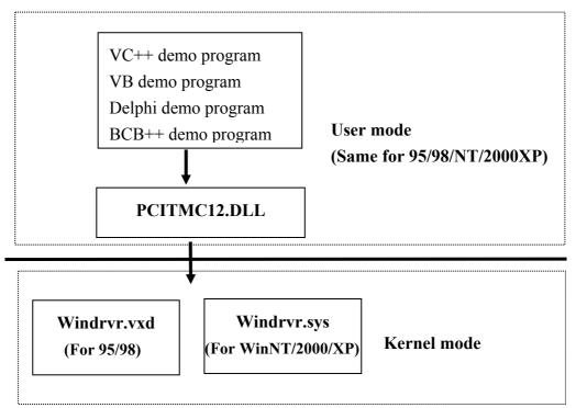
The install shield will install kernel driver, DLL driver & application demo program to system. All demo program & DLL are same for 95/98/NT/2000/XP. But the kernel drivers are different for different systems as follows:
