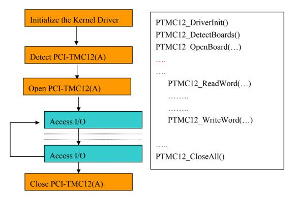
For multi-task applications, many user programs will control OME-PCI-TMC12(A). So the program will open & lock OME-PCI-TMC12(A) before access the I/O. Then un-lock OME-PCI-TMC12(A) after access the I/O as follows:
