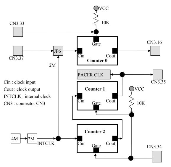
The counter0, counter1 and counter2 are all 16 bit counters. Counter 1 and counter 2 are cascaded as a 32 bit timer. This 32 bit timer is used as a <u>pacer timer</u>. The software driver, A-822\_Delay(), uses counter 0 to implement a machine independent timer for settling time delay (sec. 2.4.6 and sec. 2.4.7). If A-822\_Delay() is not used, counter0 can be used as a general purpose timer/counter.
