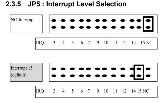
The interrupt channel <u>can not be shared.</u> The OME-A-822 software driver can support 8 different cards in one system but only **2 of these cards** can use the interrupt transfer function.
