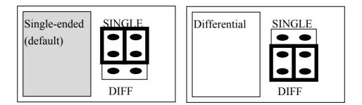
The OME-A-822PGL/PGH offers 16 single-ended or 8 differential analog input channels. The JP3 jumper sets the inputs to single-ended or differential mode. You can not select single-ended and differential simultaneously.
