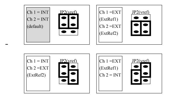
If JP2 is set to **internal reference**, then JP1 should be set to **-5V or -10V** internal reference voltage.
