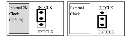
The OME-A-822PGL/PGH has 3 independent 16 bit timer/counters. The cascaded counter1 and counter2 are used as **a pacer timer**. Counter0 can be used as a user programmable timer/counter. The user programmable timer/counter can be set to **2M internal clock** or **external clock ExtCLK**, **CN3 pin 37**. The block diagram is given in section 2.6. The clock source must be very **stable**. Using the 2M internal clock is strongly suggested.
