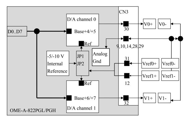
NOTE : The D/A output latch registers use a "double buffer" structure. <u>The user must</u> send the low byte data first, then send the high byte data. If the user
