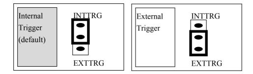
The OME-A-822PGL/PGH supports two trigger types, **internal trigger** and **external trigger**. The external trigger comes from **ExtTrg**, **CN3 pin 17**. There are two types of internal triggers, **software trigger** and **pacer trigger**. More detailed information is given in section 2.4.8.
