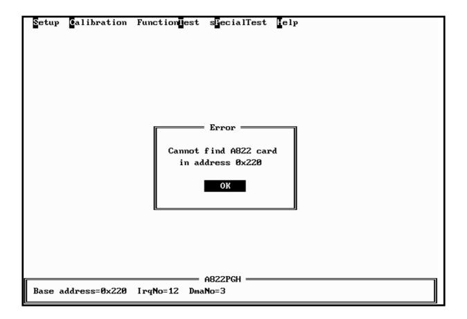
Although you can continue by pressing any key, it is recommended that the jumper situation be corrected since many operations in the A82XDIA utility check the I/O base address and report an error if the configuration file and the actual jumper settings do not match.
