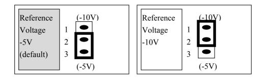
Select (-5V) : D/A voltage output = 0 to 5V (both channel) Select (-10V) : D/A voltage output = 0 to 10V (both channel) JP1 is valid only if JP2 is set to D/A internal reference voltage
