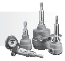
Omega's LTU-2000 Series use a piezo-electric crystal that enables the switch to vibrate at a fixed pre-defined resonant frequency. When the tuning fork is submerged in the medium the frequency at which the switch is vibrating, changes. This change is detected by the unit's electronics and is converted into a switch output (either relay or PNP/NPN depending on the model).
