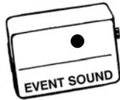
the KES will respond to very low levels of sound. In many cases the ambient noise in a small room will be sufficient to be recognized as an "ON" condition with the threshold adjustment at this setting.
