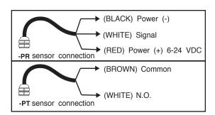
the lens. The sensor turns on and off once each time the magnet passes under it. Sensors are designed for electronic control loads, and should not be used to switch power loads or line voltages. See maximum current and voltage ratings, under Specifications.
