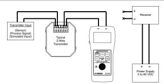
The Model CL530 supplies 24 Volts to the transmitter and displays the output in mA or % on the Model CL530 display. If the Model CL530's HART® protocol mode is selected, an internal  $250 \Omega$  load resistor is connected in series with the output as specified for proper communication by HART® devices. This eliminates the requirement of connecting a separate  $250 \Omega$  load resistor in the field as indicated in field hookup diagrams of HART® enabled devices.
