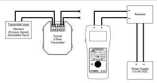
The Model CL530 can simulate a 2-wire transmitter in the 4-20 mA process loop. The calibrator will indicate "LOW SUPPLY" if improperly connected. The EZ-Check" switch and EZ-Diali" knob allow rapid and fine control of loop current. The EZ-Step" button and hands-free auto step/ramp function allow a complete check of calibration points.
