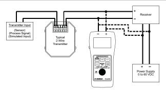
The Measure DC Volts Mode reads voltage from 0.00 to  $\pm 60.00$  VDC. This mode can be used to check loop power, measure voltage drop across  $250\Omega$  load loop resistors, 1 to 5V signals, I/V converters and battery voltages.
