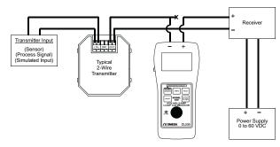
The Model CL530 can read loop currents from 0-24 mA. The Model CL530 limits current in read mode to less than 24 mA to protect the devices in the loop from over voltage or over current conditions.
